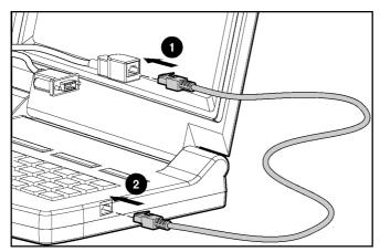
Figure 2-3: Connecting an RJ-45 network cable
